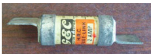
Photo 1: GEC Fuse Type NS2 – Contains asbestos
