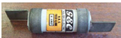
Photo 2: GEC Fuse Type NS16 – Does not contain asbestos (Note subtle variation in label design)
