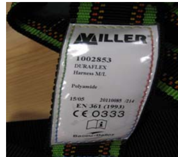
Fig 3 – This is the manufacturer's information label – note the serial number
