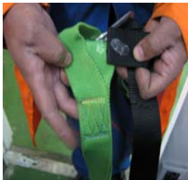
Fig 1 – This shows the defective harness with the adhesive on the harness, which should additionally have been double-stitched
