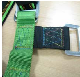
Fig 2 – This shows the correct method of attachment
