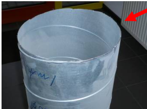
Shots show the type of ducting used clearly showing the jagged edges, which caused the cut Below is a shot of the work area.
